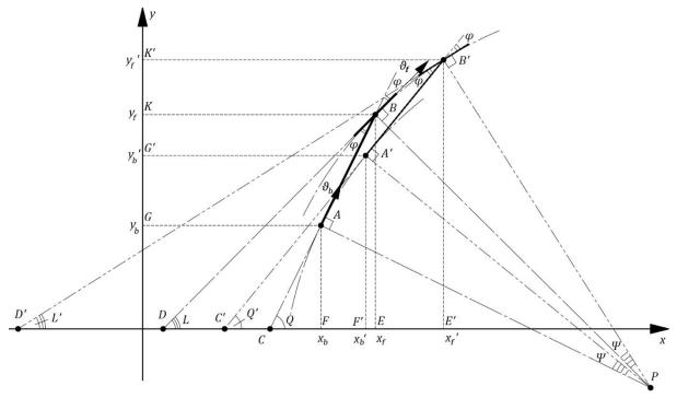
Fig. 1 Kinematic diagram of a mobile robot
